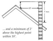
If a chimney is too short, or if the flue too large, your stove's hot exhaust can cool and reduce the "engines draft". A slow draft can lead to poor stove performance, smoke spillage, or back puffing. Generally, if the Survival Hybrid is installed with a 10-12 foot chimney and there is smoke spillage or backpuffing, the height of the chimney may have to be increased by adding another section of pipe on the outside of the home to create better flow through the stove and up the chimney.
