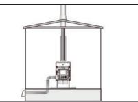
An optional outside air kit is available if the Survival Hybrid is being installed in a mobile home. The outside air kit has a 4" collar on the back of the stove. From this collar, a 4" metal duct must be installed through the floor and horizontally to the outside of the house. The termination of the duct must be covered with a screen with holes no greater than 1/4" square.
